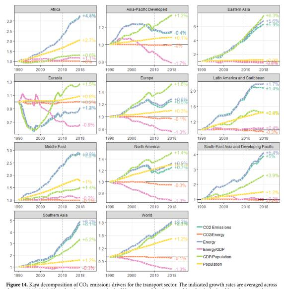
**Figure 14.** Kaya decomposition of  $CO_2$  emissions drivers for the transport sector. The indicated growth rates are averaged across the years 2010–2018. Note that the energy term by itself is not part of the decomposition, but is depicted here for comparison with the Kaya factors. This figure is for fossil fuel  $CO_2$  emissions only (indirect  $CO_2$  emissions are excluded) in order to ensure compatibility with underlying energy data.
