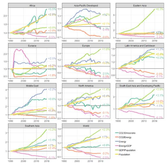
**Figure 11.** Kaya decomposition of  $CO_2$  emissions drivers for the buildings sector (direct emissions only). The indicated growth rates are averaged across the years 2010–2018. Note that the energy term by itself is not part of the decomposition, but is depicted here for comparison with the Kaya factors. This figure is for fossil fuel  $CO_2$  emissions only (indirect  $CO_2$  emissions are excluded) in order to ensure compatibility with underlying energy data.
