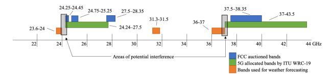
**Figure 1.** 5G band allocations of the FCC and 2019 International Telecommunication Union (ITU) World Radiocommunication Conference (WRC-19) compared to existing spectra used for weather prediction. Image credit: Shantam Rayan.
