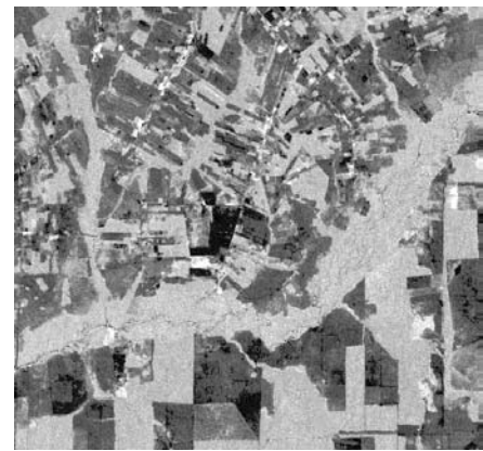
Fig. (16d). Zoom of a continuous greenness index change ( \Delta GR ) image where: (i) \Delta GR < 0 if ( GR2 < GR1 ); (ii) \Delta GR > 0 if ( GR2 > GR1 ); and (iii) dumb negative value ( = -150 ) if ( (GR1 == 0) \text{ AND } (GR2 == 0) ), equivalent to the “never vegetation” condition.
