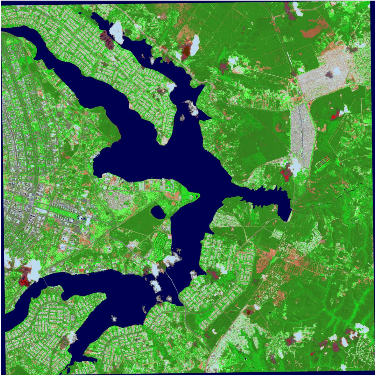
Fig. (12). I-SIAM™ preliminary map of the QuickBird-2 image shown in Fig. (11). Spectral categories are depicted in pseudo colors. Map legend: refer to Table 5 (for interpretation of the references to color in this figure caption, the reader is referred to the web version of this paper).
