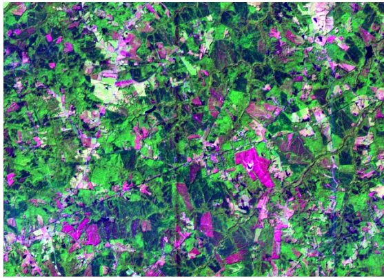
Fig. (15a). Zoomed area of a Landsat 7 ETM+ image of Virginia, USA (path: 16, row: 34, acquisition date: 2002-09-13), depicted in false colors (R: band ETM5, G: band ETM4, B: band ETM1), 30 m resolution, radiometrically calibrated into TOARF values (for interpretation of the references to color in this figure caption, the reader is referred to the web version of this paper).
