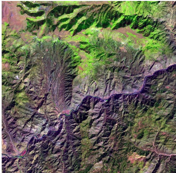
Fig. (13a). Zoomed area of a Landsat 7 ETM+ image of Colorado, USA (path: 128, row: 021, acquisition date: 2000-08-09), depicted in false colors (R: band ETM5, G: band ETM4, B: band ETM1), 30m resolution, radiometrically calibrated into TOARF values (for interpretation of the references to color in this figure caption, the reader is referred to the web version of this paper).
