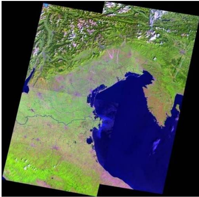
Fig. (14a). Mosaic of four radiometrically calibrated Landsat 7 ETM+ images: Emilia-Romagna, Veneto, Friuli regions in Northern Italy. Spatial resolution: 30 m. An image boundary effect is clearly visible (for interpretation of the references to color in this figure caption, the reader is referred to the web version of this paper).
