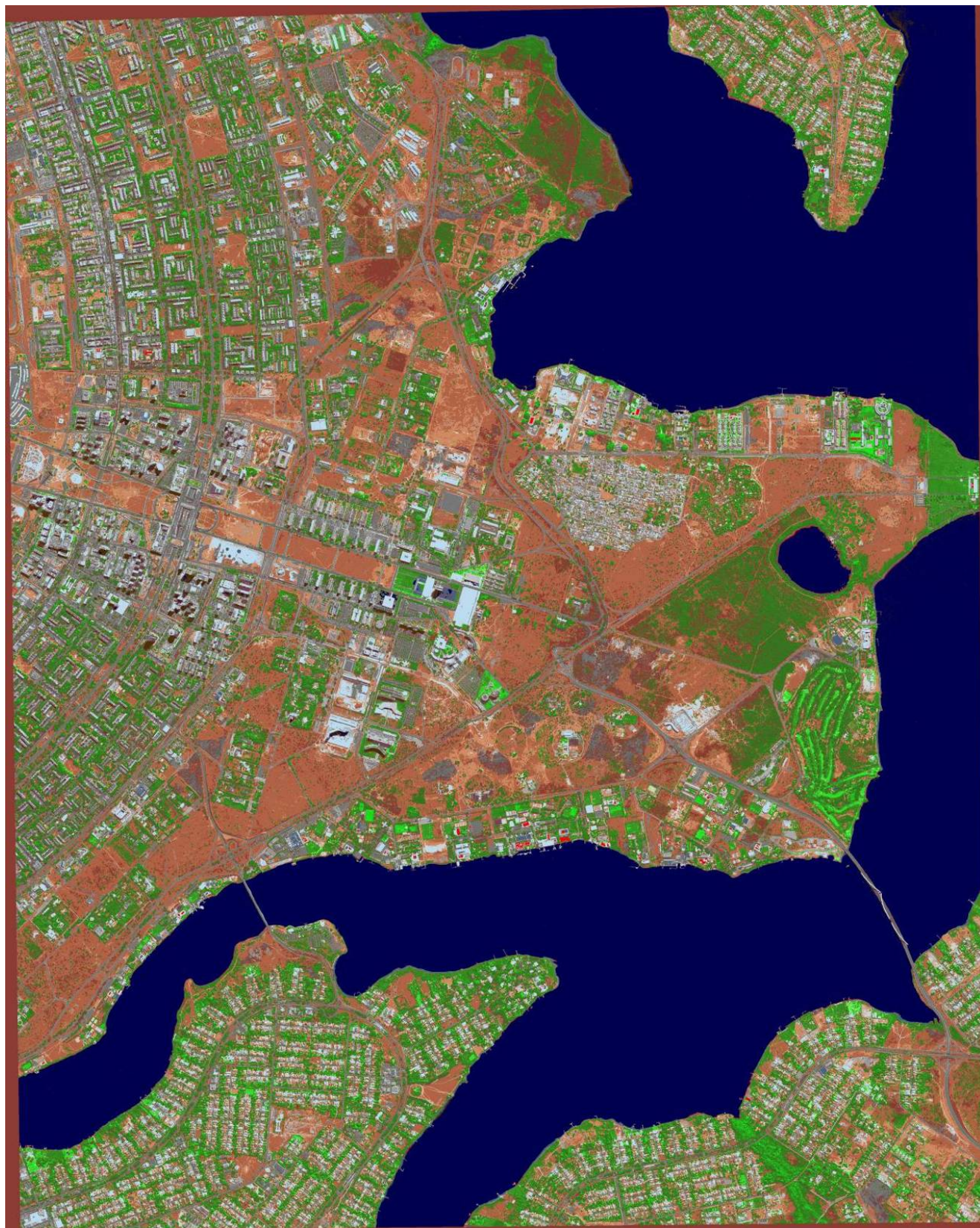
Fig. (10). I-SIAM™ preliminary map of the WorldView-2 image shown in Fig. (9). Spectral categories are depicted in pseudo colors. Map legend: refer to Table 5 (for interpretation of the references to color in this figure caption, the reader is referred to the web version of this paper).
