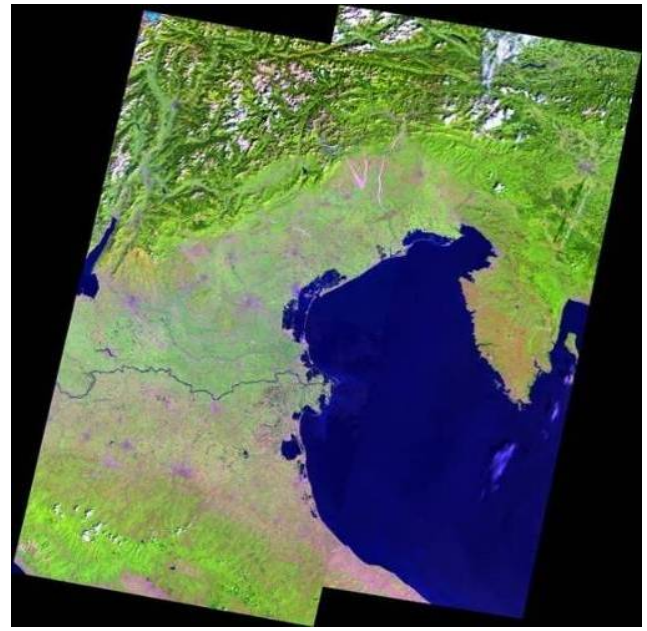
Fig. (14c). Mosaic of the four radiometrically calibrated Landsat 7 ETM+ images shown in Fig. (14a) after semantic-driven (stratified) histogram matching between a “master” image (say, Veneto) and the remaining “slave” images (Emilia-Romagna and Friuli). No image boundary effect is now visible (for interpretation of the references to color in this figure caption, the reader is referred to the web version of this paper).
