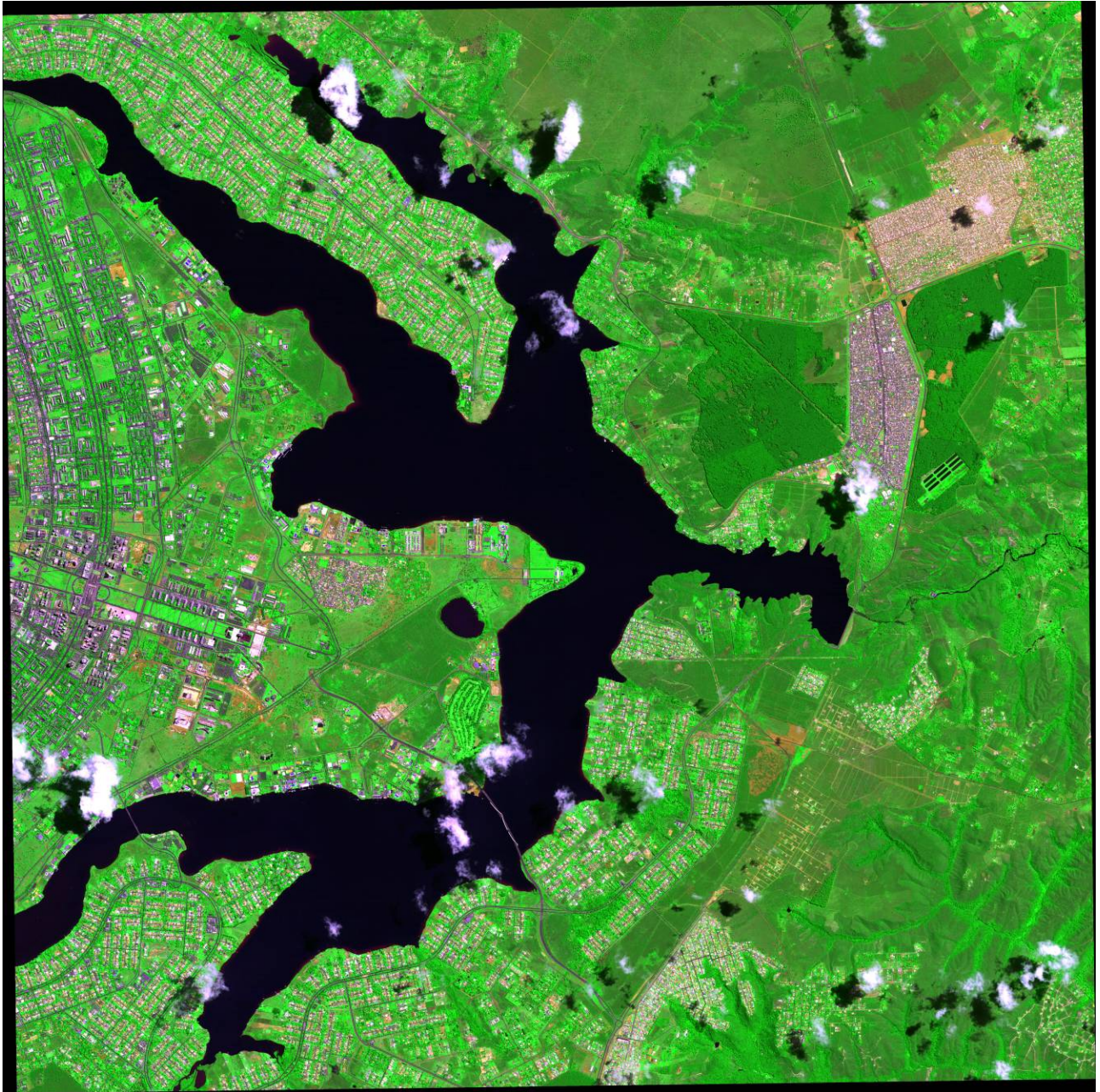
Fig. (11). 4-band QuickBird-2 VHR image of the city area of Brazilia, Brazil, acquired on 2010-03-16, at 13:25 GMT, depicted in false colors (R: band R, G: band NIR1; B: band B) (provided by Digitalglobe, 8-band Challenge), radiometrically calibrated into TOARF values. Spatial resolution: 2.4 m (for interpretation of the references to color in this figure caption, the reader is referred to the web version of this paper).
