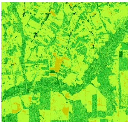
Fig. (16c). Zoom of a Bi-Temporal change detection map generated from the preliminary classification map pair shown in Fig. (16a) and Fig. (16b). Change/no-change map legend: refer to Table 7 (for interpretation of the references to color in this figure caption, the reader is referred to the web version of this paper).
