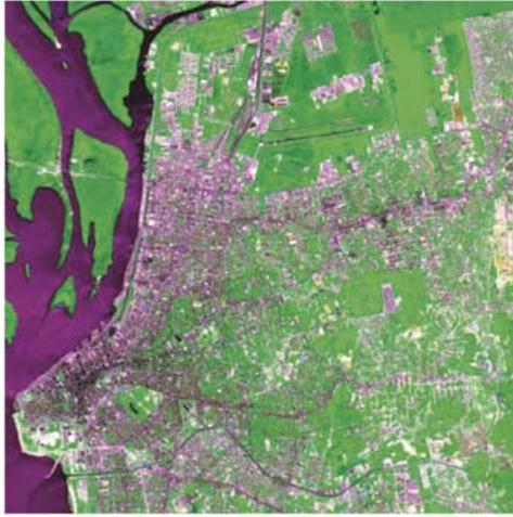
Fig. 6. Test case 1. False-color composition (B: VisBlue, G: NearIR, R: VisRed) of the SPOT image of Porto Alegre, Brazil,  $512 \times 512$  pixels in size, three-band, 20-m spatial resolution, acquired on November 7, 1987.
