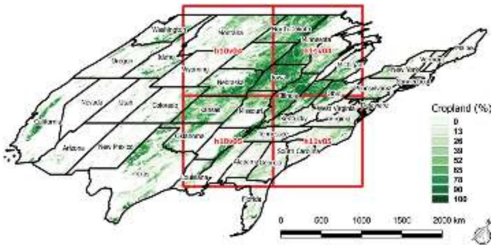
**Figure 2.** Illustration of four MODIS tiles over the United States (in MODIS sinusoidal projection) used for comparison of 500 m 8-day composite products from MODIS (MYD09A1) and VIIRS (VNP09A1) sensors. Shown in green also is a distribution of croplands derived from the USDA's Cropland Data Layer (CDL) for 2016 (Johnson and Mueller 2010) and averaged to CMG (0.05°) scale.
