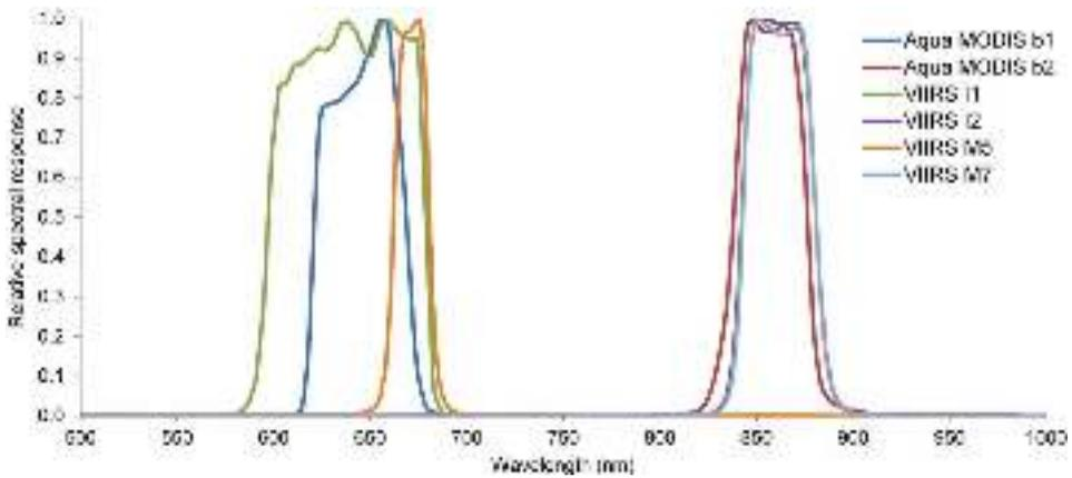
**Figure 1.** Relative spectral response functions for MODIS/Aqua and VIIRS sensors in the red and NIR spectral domain. The functions for MODIS and VIIRS were derived from <https://mcst.gsfc.nasa.gov/calibration/parameters> and <https://ncc.nesdis.noaa.gov/VIIRS/VIIRSSpectralResponseFunctions.php>, respectively.
