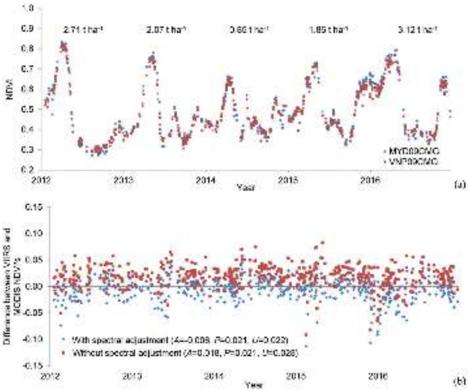
**Figure 11.** A time series of NDVI values derived from BRDF-corrected MYD09CMG and VNP09CMG daily products at 0.05° resolution for Harper County. SR values in red (I1) and NIR (I2) bands that were used to compute NDVI from VIIRS were spectrally adjusted to match the MODIS/Aqua ones. Shown also are final winter wheat yields derived from USDA NASS statistics (a). A difference between aggregated NDVI values from MYD09CMG and VNP09CMG with and without spectral adjustment for VIIRS bands (b).
